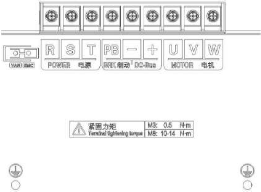
Fig. 3-3 380V 30-75kW, 660V 18-30 and 75-90kW main circuit terminals (the -3/-6 series have no PB terminal)
