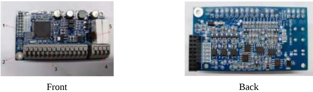
Fig. 9-3 Picture of a real IO expansion card
