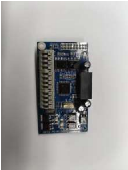
Fig. 9-20 Rotary transformer PG card - real product
